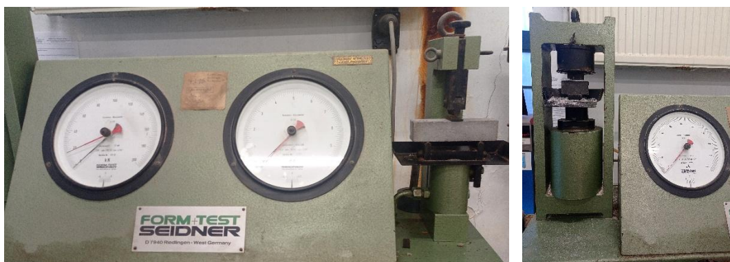
Fig. 4. Flexural strength tests conducted to determine pozzolanic properties.
