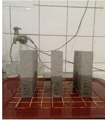
Fig. 8. Capillary water absorption test setup.
