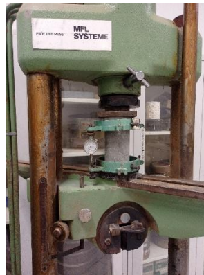
Fig. 7. Static elasticity modulus test setup.
