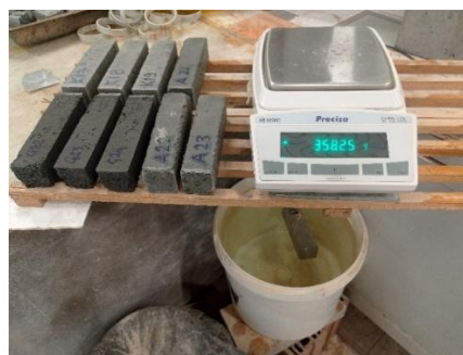
Fig. 9. Water absorption by weight and visible porosity test setup.
