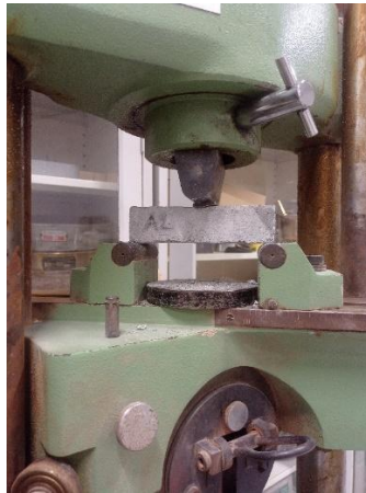
Fig. 5. 100 kN capacity testing machine used for the flexural strength test.
