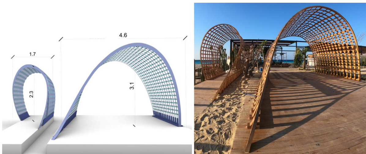
Fig. 6. on the left side the initial design for the prototype and on the right side the executed one (Author, 2025).
