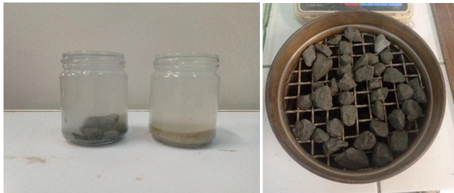
Fig. 1. Specific gravity and sieve analysis of aggregates
