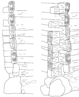
Fig. 2. Drawing of rectangular section kurtboğaz technique (Halı Kabataş ve Sağiroğlu, 2021)
