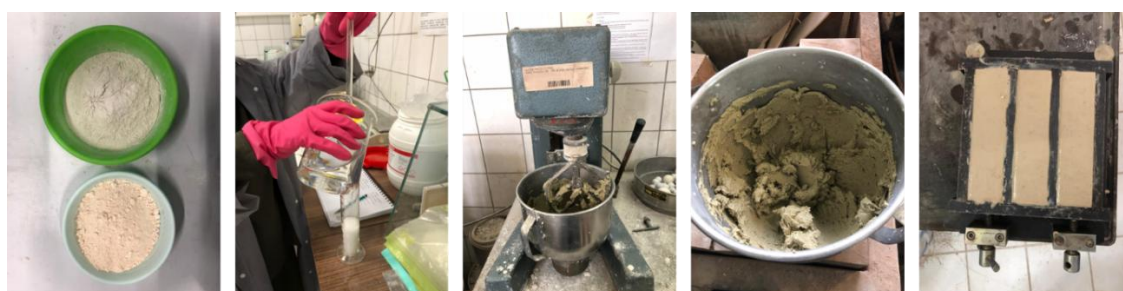
Fig. 1. Production stages of geopolymer binders
