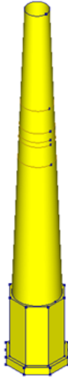
Fig.6. Model of chimney after strengthening with rings at one-third of the chimney's height from the top
