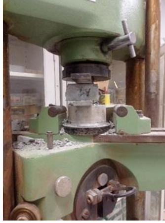
Fig. 6. 100 kN capacity testing machine used for the compressive strength test.
